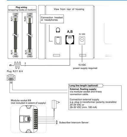
**Note:** The connection for an external loudspeaker can be switched to an input or open-collector output via internal jumper (output relay retrofittable).
